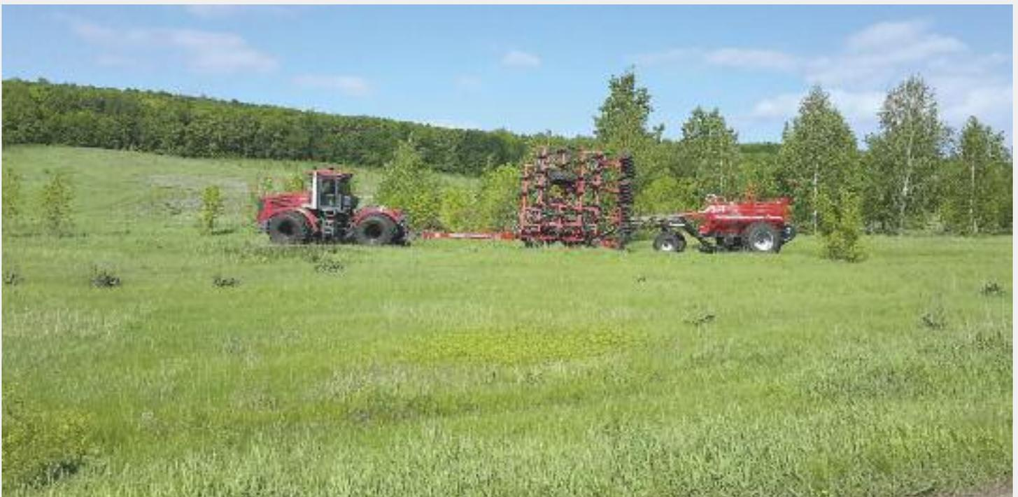
*A powerful combination: the newly acquired 420 hp Kirovets tractor pulls the 12 m Kverneland no-till seeder with a 8,000 l seed and fertilizer bunker. Tractor and seed-combination are produced in Lipetsk, Russia*
