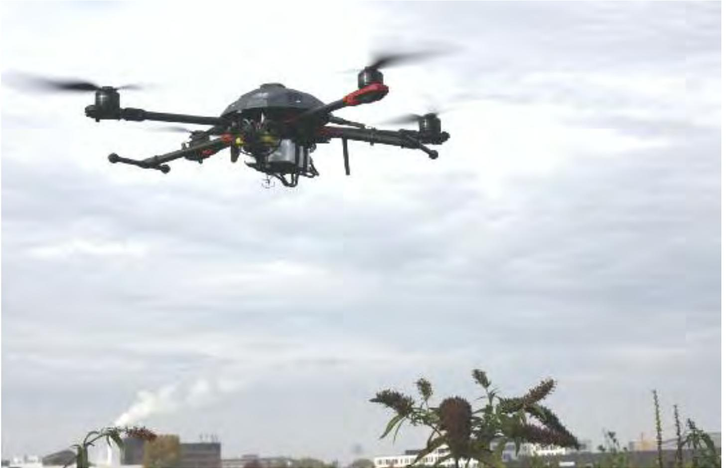
AHT's new Unmanned Aerial Vehicle (UAV) equipped with an optical sensor (digital camera), a video camera, an autopilot system and a GPS navigation system during a test flight over a fallow near Essen. With the termination of the testing phase AHT is ready to deploy its
