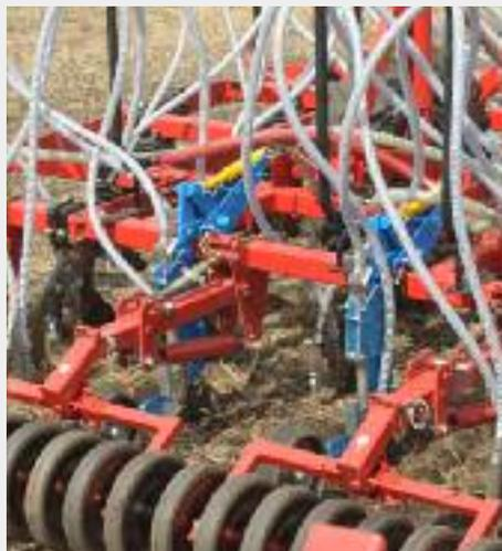
*Two Primary precision seeder tines (blue) mounted on a 12 m Kverneland air seeder*
